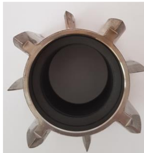
Extruder with Carbon Bearing Pressed Into Place
